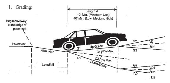
The shoulder slope usually varies from 1/8"/ft. (2%) to 3/4"/ft. (6%). However, the shoulder slope should be maintained when constructing the driveway.
